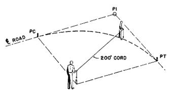
Figure 3. A curve staked by using a cord.
