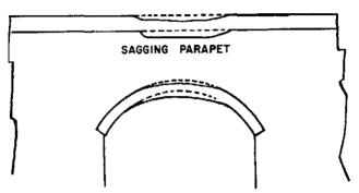
Figure 117. Deformation of arch ring.
