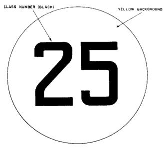
Figure 48. Example of vehicle classification sign.
