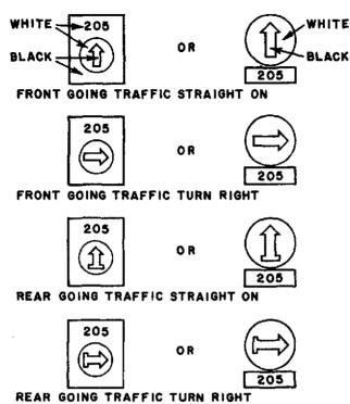
Figure 42. Examples of guide signs for specific axial military routes.
