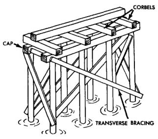
Figure 98. Timber pile pier.
