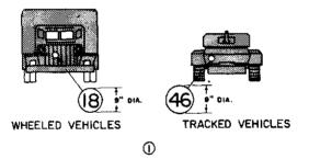
Figure 49. Markings and typical locations of classification signs for single vehicles.
