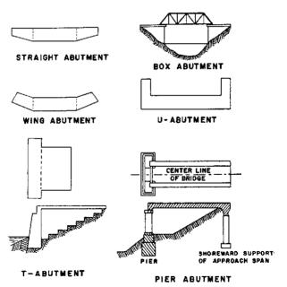
Figure 104. Common types of abutments.
