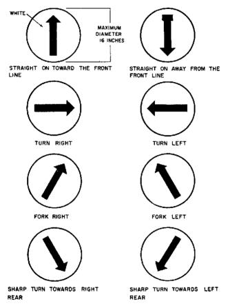
Figure 46. Examples of directional disks.
