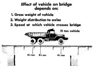
Figure 25. Effect of vehicle on bridge.
