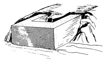
Figure 107. Typical U-type abutment.
