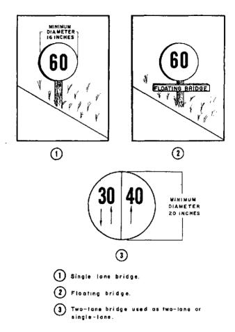
Figure 34. Typical bridge class and information signs.
