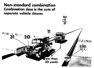
Figure 27. Nonstandard combination of vehicles.
