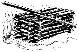
Figure 99. Typical crib pier.
