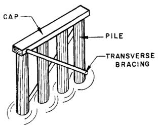
Figure 94. Pile bent.
