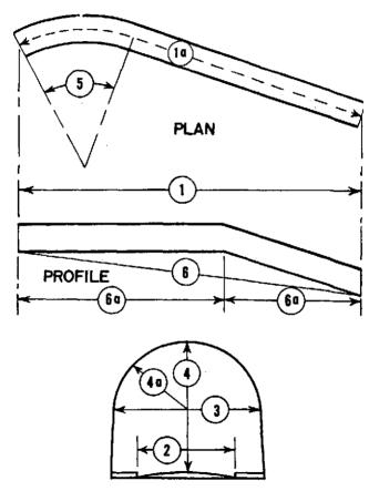
Figure 13. Standard dimensional data for tunnels.
