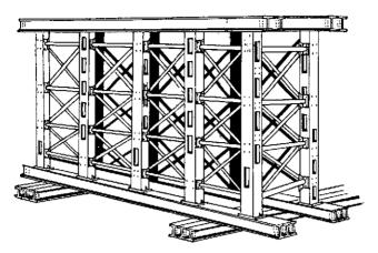
Figure 101. Typical prefabricated steel trestle pier.
