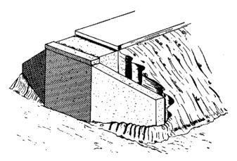
Figure 108. Typical wing type abutment.
