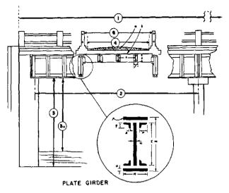
Figure 77. Standard dimension data for plate girder bridges.
