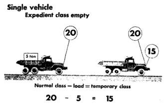
Figure 29. Example of classification of an empty vehicle.
