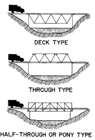
Figure 71. Classification of truss types by position of roadway.
