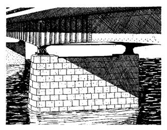
Figure 100. Typical masonry pier.
