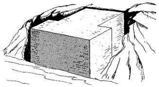
Figure 106. Typical T-type abutment.
