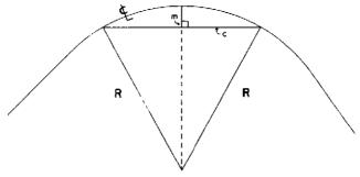
Figure 5. Measuring a curve using formula  $R = C^2/8m + m/2.$
