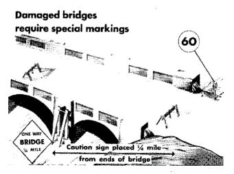
Figure 20. Example of damaged bridge.
