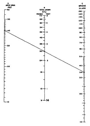
Figure 112. Alinement chart for determining the provisional load classification of masonry arch bridges.
