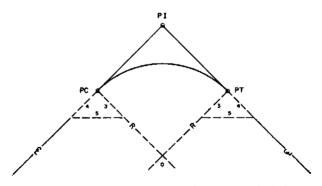
Figure 4. Curve radius by locating center of circle.
