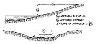
Figure 14. Standard dimensional data for fords.
