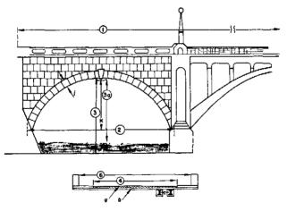
Figure 80. Standard dimension data guide for arch bridges.
