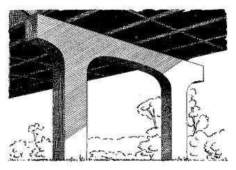
Figure 102. Typical open type concrete pier.
