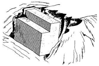
Figure 105. Typical straight abutment.
