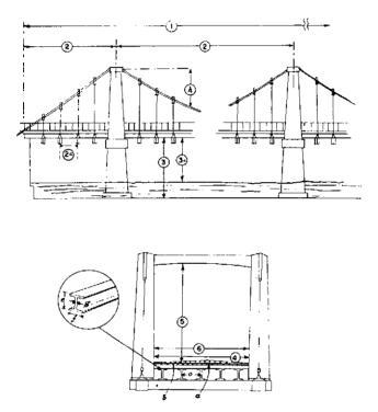
Figure 89. Standard dimension data guide for suspension bridges.
