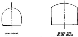
Figure 118. Common types of tunnel bores or cross sections.
